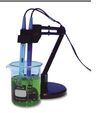
Model SH300 holds up to three standard electrodes.
