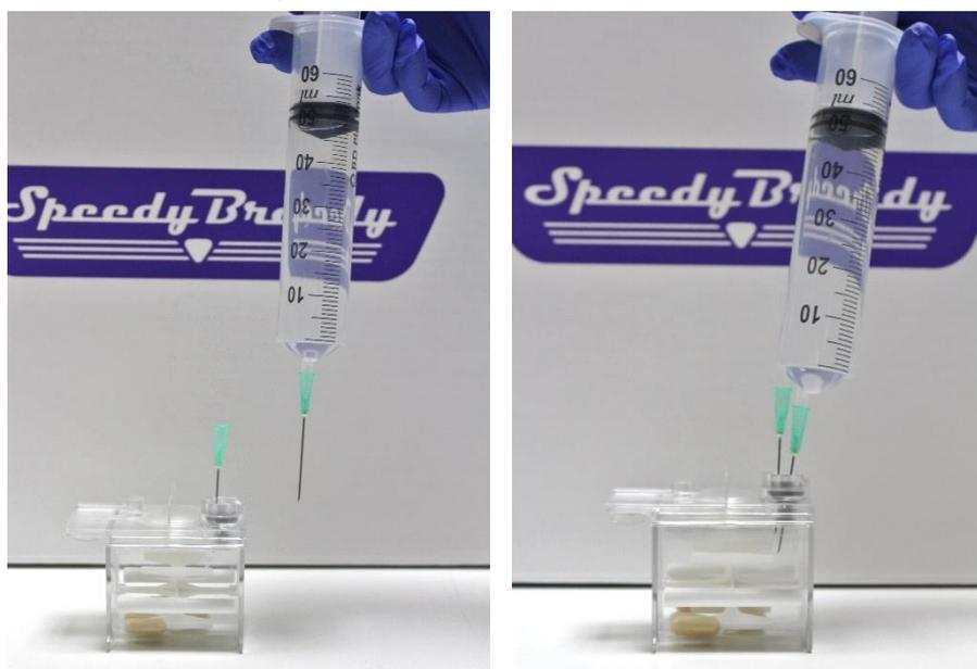
Figure 6: Adding a sample through the self-sealing rubber.
